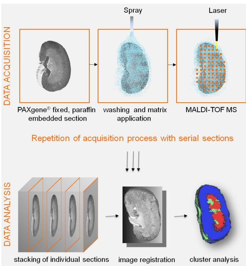
FIG. 2 Experimental and computational pipeline for 3D MALDI-IMS of a mouse kidney
